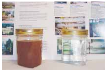
Within a few weeks of installing the pulsed-power water treatment system, the process water at the Dow Chemical Technology Center changed from a murky greenish brown to crystal clear.
