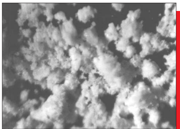
Figure 4b - Bulk-Solution Precipitate 60x • Pulsed-Power Treatment •
